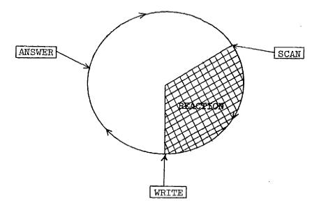
The computer ("central processing unit") does all its work in the shaded part of the diagram, in the space of, say, 1/1000 second. The solid line represents the stone carver at work, hacking out the display at the rate of 250 characters per second. The unshaded part represents the student's reaction, occupying 10, 15, 30 seconds or more...however long it takes him to read what has been written for him on the screen, to type in something new, and to push the "send" button.
